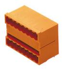
2-tier male connector with parallel pin arrangement. The solder pin length is optimised for wave flow soldering. The male connectors provide space for labelling and can be coded. Packed in cardboard box.
