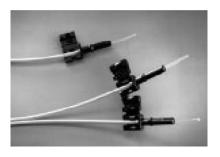
To install simplex connectors flip the top half of the connector over and snap it into the ferrule half (with your fingers). When the top half latches inside the body of the ferrule half, proper connector-to-cable attachment is achieved.
