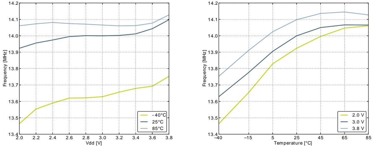
**Figure 3.25. Calibrated HFRCO 21 MHz Band Frequency vs Supply Voltage and Temperature**
