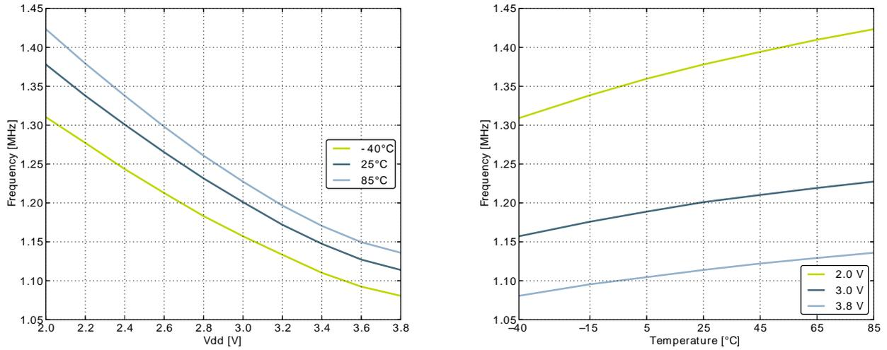
**Figure 3.22. Calibrated HFRCO 7 MHz Band Frequency vs Supply Voltage and Temperature**
