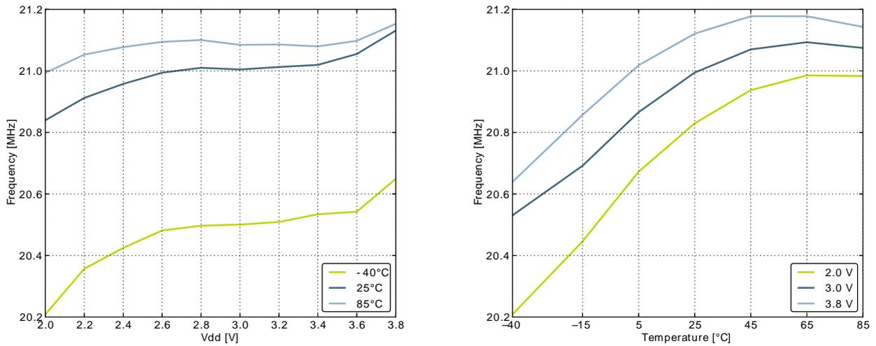
**Figure 3.26. Calibrated HFRCO 28 MHz Band Frequency vs Supply Voltage and Temperature**
