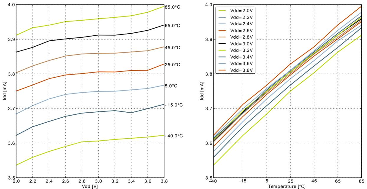
**Figure 3.3. EM0 Current consumption while executing prime number calculation code from flash with HFRCO running at 14 MHz**
