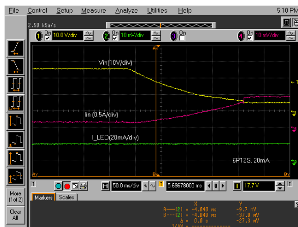
FIGURE 15. LINE REGULATION WITH V_{IN} CHANGE FROM 26V TO 6V FOR 4P12S AT 20mA/CHANNEL
