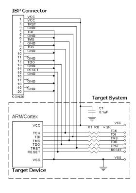
Powering the target device: There are two alternative options for powering the targets:
