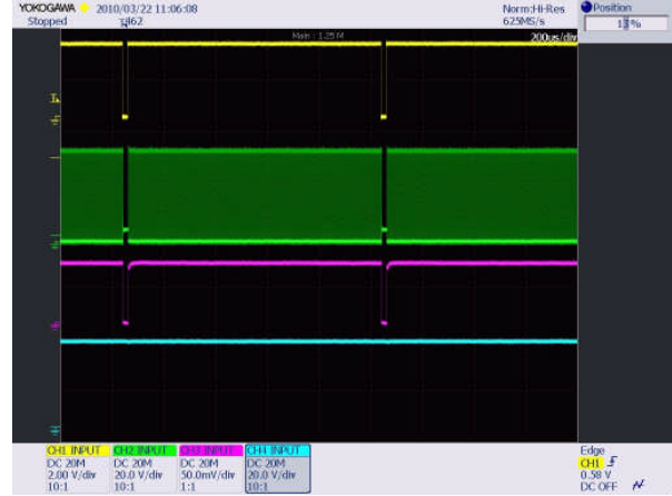
Ch 1 (yellow) – PWM signal at 1 kHz 98% duty cycle C2 (green) – SW node voltage, Ch 3(red) – LED Current. Ch4 (blue) - V_{OUT}
