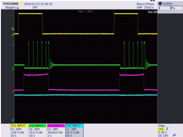
Ch 1 (yellow) – PWM signal at 30 kHz 25% duty cycle C2 (green) – SW node voltage, Ch 3(red) – LED Current. Ch4 (blue) - V_{OUT}
