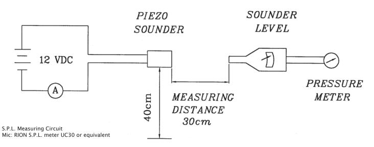
2) The current consumption and the sound pressure level are measured by using the recommended driving circuit as shown below.
