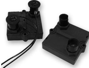
With a maximum inductance of 80nH and a rated power of 600W (60°C Heatsink) in a 57mm x 60mm casing, the BDS600 offers high power density over a wide range of ohmic values (0R5 – 100K).
