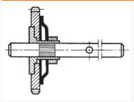
This device is situated inside the gearbox and is particularly recommended when gearbox protection is required in the event of accidental overloading. In this system, the final gear is connected to the gearbox output shaft by means of a friction assembly. In some cases, this device can be used for time adjustment or zero reset on timers.
