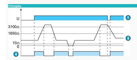
The relay is reset either using the RESET pushbutton on the front face or by opening the external contact S2 (remote reset), or by cutting the auxiliary power supply (terminals A1 - A2). If the auxiliary power is cut for a period of time greater than the reset time (500 ms), the relay is reactivated if the proble detects a normal temperature when the power supply voltage is restored.
