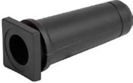
4311.0053 PVC Strain Relief for cable outside diameter 8.7mm, 3 x 16AWG
