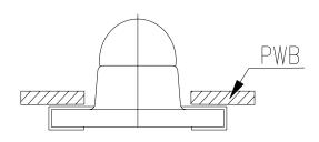
For Reflow Soldering (Propose)
