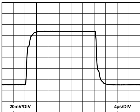
Figure 52. Small Signal Pulse Response, R_L = 10\text{ k}\Omega , C_L = 100\text{ pF} , G = 10
