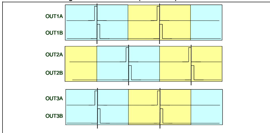
Figure 18. 2.1 channels (OCFG = 10) PWM slots
