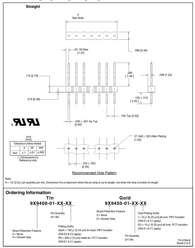
Datasheet of 929450-01-16-EU - CONN HEADER 16POS STR .100" GOLD Contact us: sales@integrated-circuit.com Website: www.integrated-circuit.com
