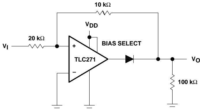
NOTE A:  $V_{DD} = 5 \text{ V to } 16 \text{ V}$
