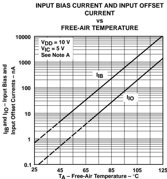
NOTE A: The typical values of input bias current and input offset current below 5 pA were determined mathematically.
