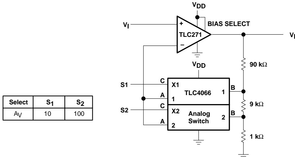
NOTE A:  $V_{DD} = 5 \text{ V to } 12 \text{ V}$
