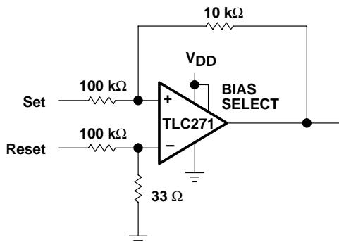
NOTE A:  $V_{DD} = 5 \text{ V to } 16 \text{ V}$
