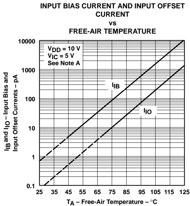
NOTE A: The typical values of input bias current and input offset current below 5 pA were determined mathematically.
