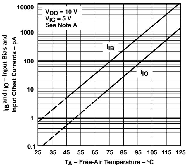
NOTE A: The typical values of input bias current and input offset current below 5 pA were determined mathematically.
