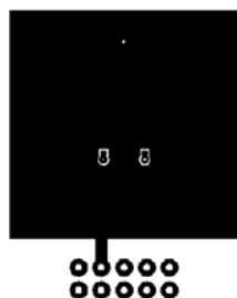
a) 40^\circ\text{C/W} when mounted on a 1 in 2 pad of 2 oz copper
