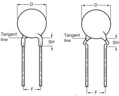
Capacitors with 10 mm (0.40") lead spacing
