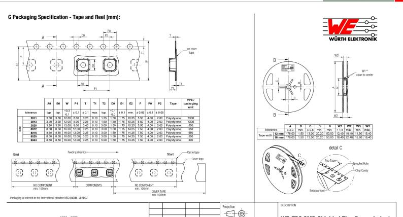
Würth Elektronik elSos GmbH & Co. KG EMC & Inductive Solutions Max-Eyth-Str. 1 74638 Waldenburg Germany Tel. +49 (0) 79 42 945 - 0 COMPLIANT ROHS&REACH WÜRTH ELEKTRONIK 2014-04-01 SSt SSt SIZE Pull-of force SSt 2013-04-08 COt Tape width 12 mm 0,1 N - 1,0 N 16 mm 0,1 N - 1,3 N 74402900016 CZ 1.0 2011-08-05 DATE CHECKED
