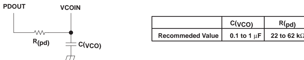
Figure 8. Resistor and Capacitor Connection
