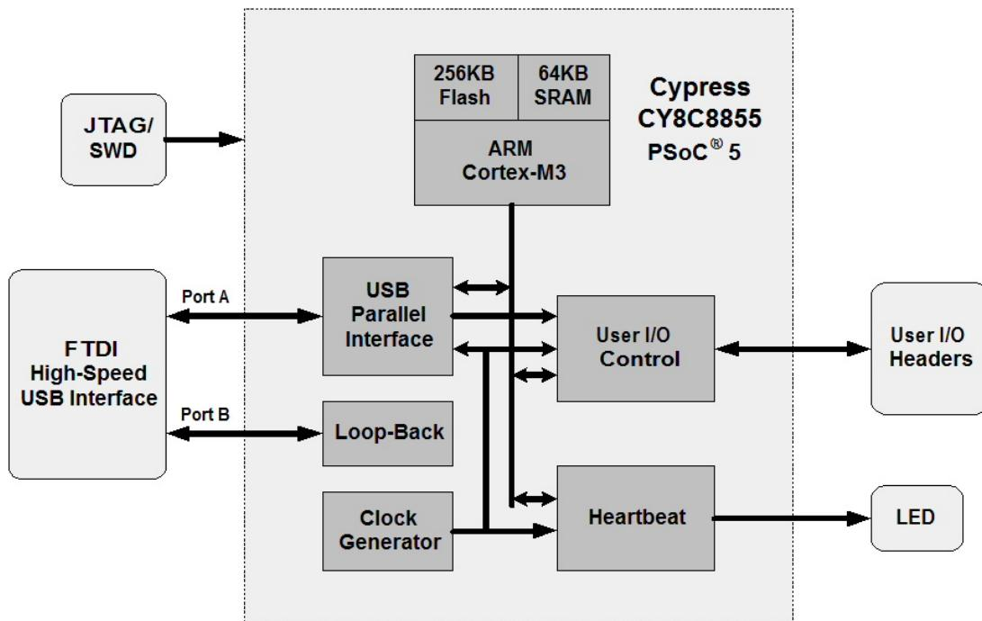
It contains the ARM Cortex M-3 CPU along with its internal memory, a USB Interface Block, a User I/O Block, a Heartbeat Pulse Generator and a Clock Generator. The JTAG Port is used to program and debug the PSoC® 5. The ARM core source code is written in C, and uses the compiler included with the PSoC Creator™ tool. The hardware implemented in the PLD blocks was created using the Cypress Component Catalog and compiled using the synthesis tool also included in the PSoC Creator™ tool.
