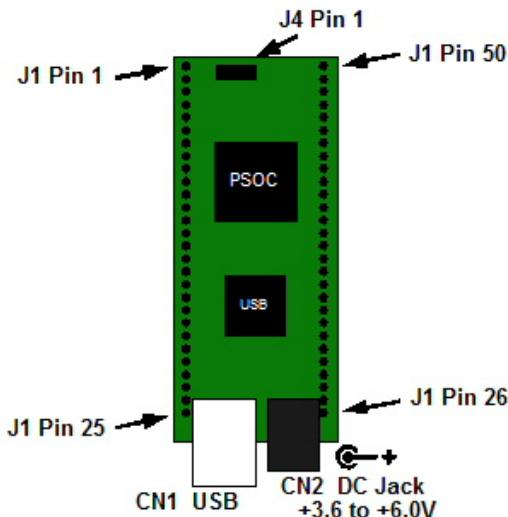
Connect the DLP-2232H-PSOC5 to the PC to initiate the loading of USB drivers. Once the USB drivers are loaded, the DLP-2232H-PSOC5 is ready for use. All commands are issued as multi-byte command packets consisting of at least two bytes.
