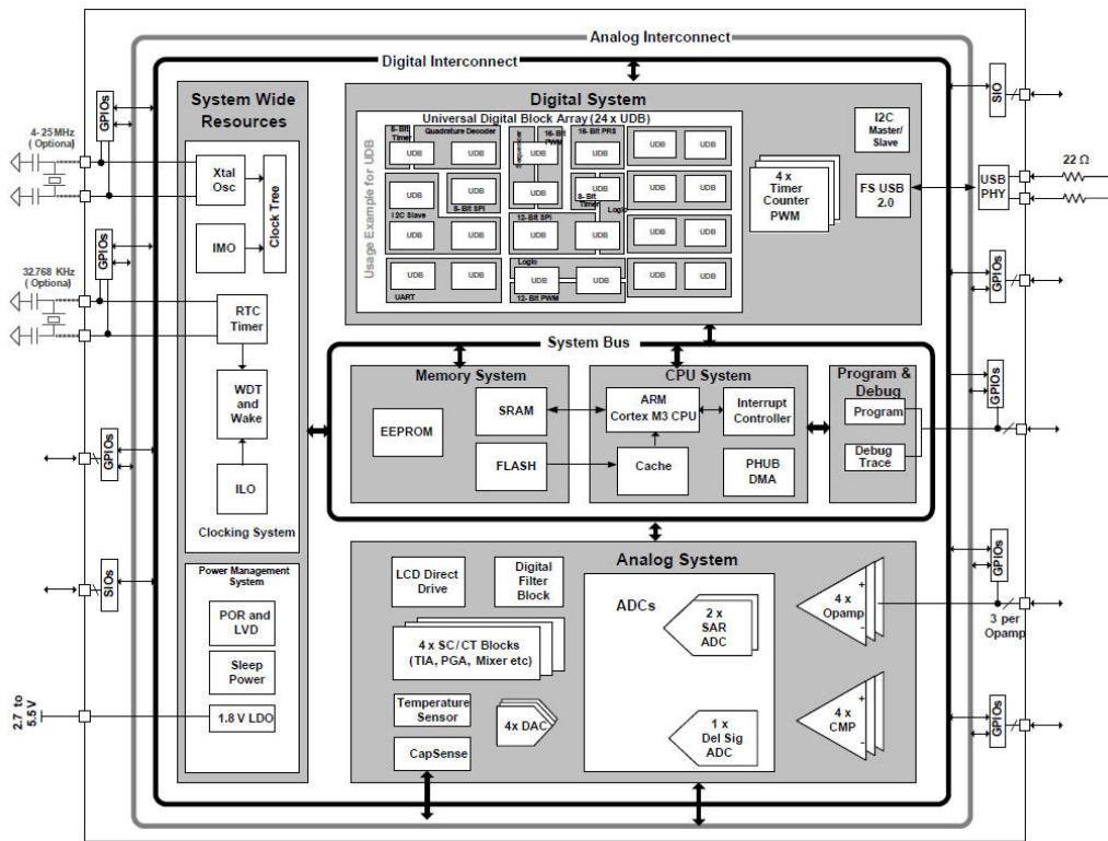
**The device used on the DLP-2232H-PSOC5 is the Cypress PSoC® 5 CY8C5588AXI-060. It contains the following:**
