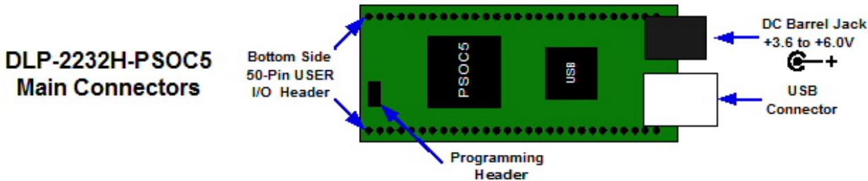
Connection to user electronics is made via a 50-pin, 0.9-inch wide, industry-standard 0.025-square inch post DIP header on the bottom of the board. The bottom side 50-pin header provides access to the user input/output pins as well as the USB port power output and the module's power input. The bottom side header mates with a user-supplied, standard, 50-pin, 0.9-inch spaced DIP socket.
