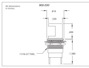
These Chicago Miniature Lamp Instrument Lites are specifically designed to provide localized light for illuminating panels, meters, switches and legends. Two sizes are available to suit your specific illumination requirements. Both units feature highly reflective surfaces on the inside of their hoods to assure peak light output and are easily relamped from the front of the panel. The lamp is not included with this indicator light; please order the required lamp separately.
