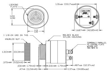
NOTE AF TERMINALS-032 BRASS TIN PLATED, TAPPED FOR #6-32 SCREW, TWO #6-32 NICKEL PLATED BRASS SCREWS INCLUDED. WILL ACCEPT 1/4" QUICK CONNECT. NOTE B: MOUNTING- REMOVE BLACK PLASTIC NUT AND INSERT THREADED FRONT THROUGH 1.25' HOLE PUNCHED IN PANEL, IF DRIENTATION IS NEEDED, NOTE LOCKING FLATS ON DRAWING, SCREW NUT BACK ON. DO NOT OVERTIGHTEN.
