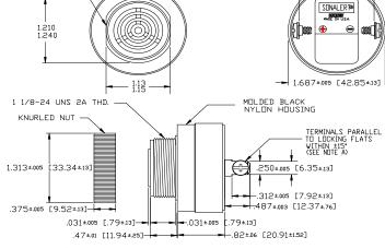
NOTE A: TERMINALS-.032 BRASS TIN PLATED, TAPPED FOR #6-32 SCREW. TWO #6-32 NICKEL PLATED BRASS SCREWS INCLUDED. WILL ACCEPT 1/47 QUICK CONNECT. NOTE B: MOUNTING- REMOVE BLACK PLASTIC NUT AND INSERT THREADED FRONT THROUGH 1.25' HOLE PUNCHED IN PANEL, IF ORIENTATION IS NEEDED, NOTE LOCKING FLATS ON DRAWING. SCREW NUT BACK ON. DO NOT OVERTIGHTEN. NOTE A: TERMINALS-.032 BRASS TIN
