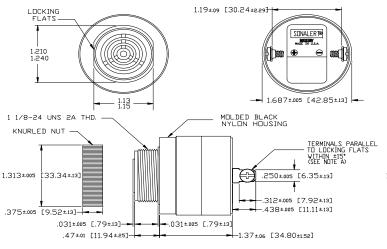
NOTE A: TERMINALS-.032 BRASS TIN PLATED, TAPPED FOR #6-32 SCREW. TVOI #6-32 NICKEL PLATED BRASS SCREWS INCLUDED. WILL ACCEPT 1/4' QUICK CONNECT. NOTE B: MOUNTING- REMOVE BLACK PLASTIC NUT AND INSERT THREADED FRONT THROUGH 1.25' HOLE PUNCHED IN PANEL, IF DRIENTATION IS NEEDED, NOTE LOCKING FLATS ON DRAWING. SCREW NUT BACK ON. DO NOT OVERTIGHTEN.
