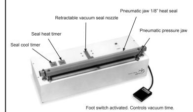
The SCS Vacuum Sealer removes moisture laden air from the interior of moisture barrier bags, and heat seals the bags closed. This is part of the dry packaging process that protects surface mount devices from moisture. A vacuum sealer, a moisture barrier bag, desiccant, and humidity indicator card (HIC) are needed for
