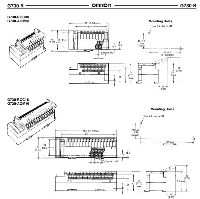
Datasheet of G730-AOM08-B DC24 - OUTPUT MODULE 8 SOLID STATE
