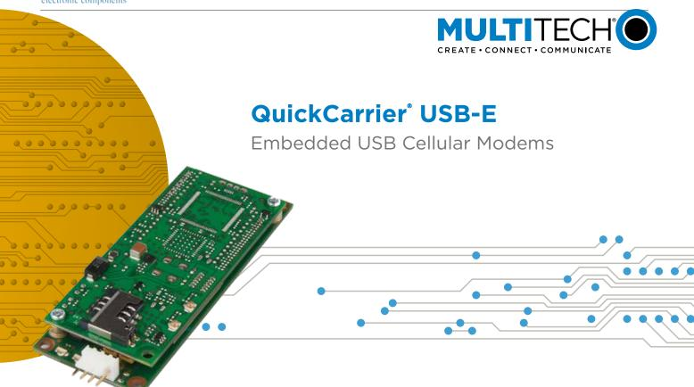
The QuickCarrier® USB-E embedded cellular modems are complete, ready-to-integrate communications devices that offer 2G and 3G cellular connectivity options. These quickto-market devices combine a network approved cellular SocketModem® and a USB carrier card in one compact design. Connectivity is easy via a 4-pin USB interface.
