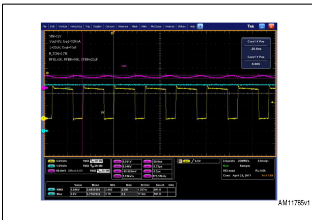
Figure 28. Load step = 0 to 300 mA
