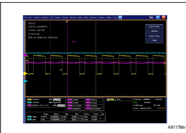
Figure 27. Load = 300 mA. Switching frequency = 410 kHz
