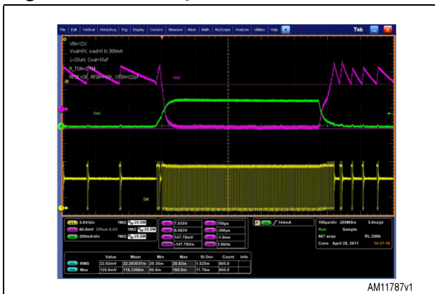
Figure 28. Load step = 0 to 300 mA
