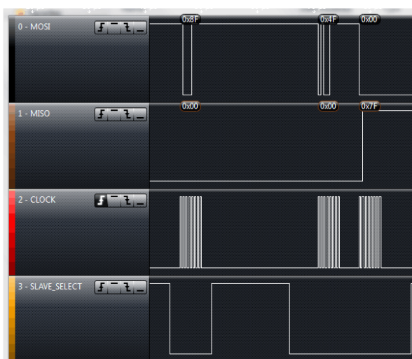
Figure 6-26. Reset FIFO and Read RSSI
