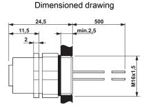
M12 flush-type socket, can be positioned
