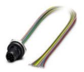
Sensor/Actuator flush-type connector, male, 8-pos., M12, A-coded, front/screw mounting with M16 thread, with 0.5 m TPE litz wire, 8 x 0.25 mm<sup>2</sup>
