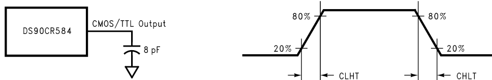
Figure 6. DS90CR584 (Receiver) CMOS/TTL Output Load and Transition Times
