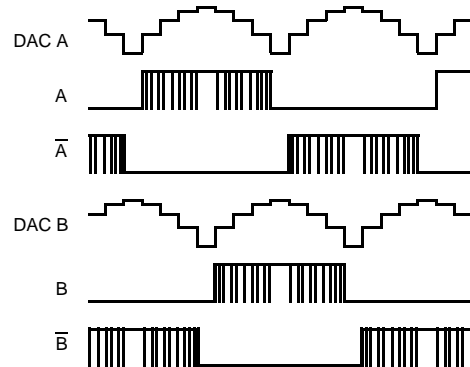
Figure 11: Stepper Motor Waveform - LM9832 Signals
