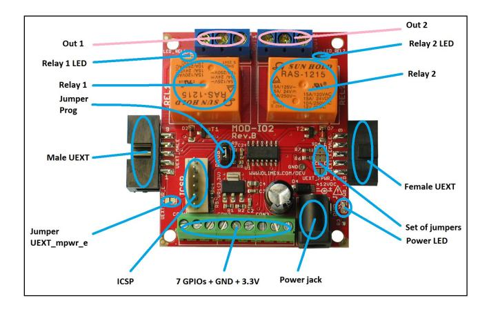
Datasheet of MOD-IO2 - MODULE GPIO AND RELAY UEXT
