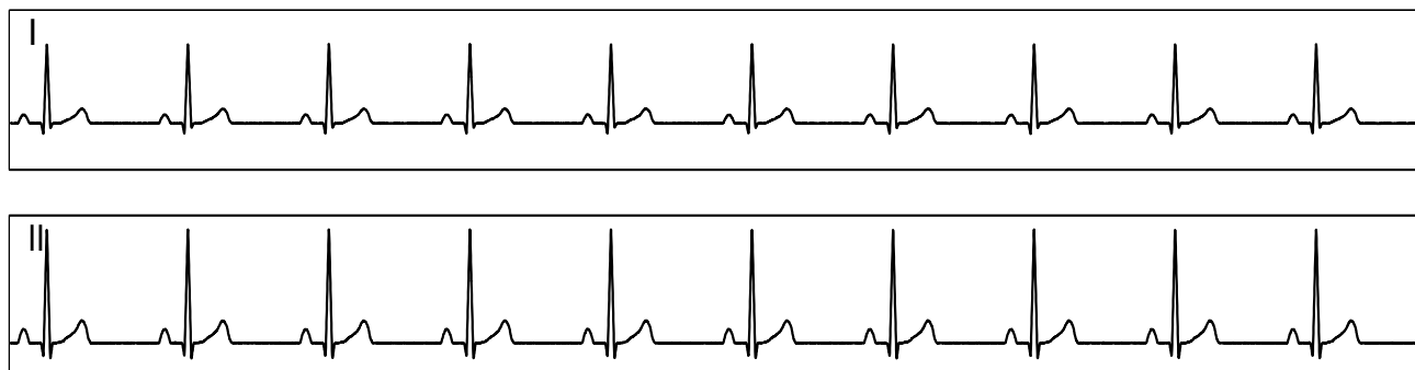
Figure 85. Single ADS1293 Device With an ECG Simulator, CH1 and CH2: ECG Signals
