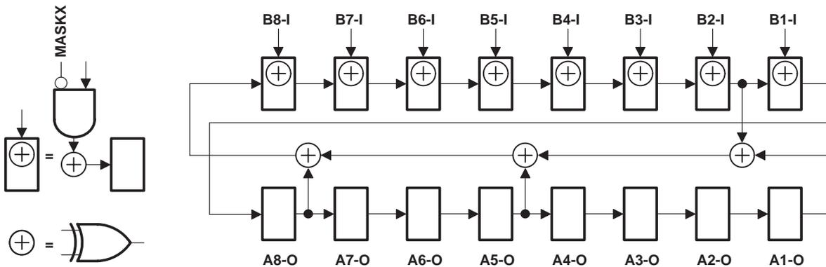
Figure 8. 16-Bit PSA Configuration (OEAB = 0, OEBA = 0)
