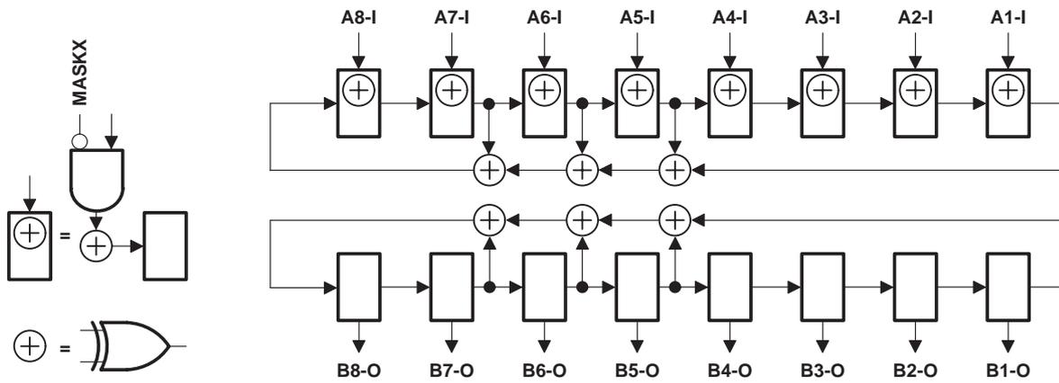
Figure 9. 8-Bit PSA/PRPG Configuration (OEAB = 1, OEBA = 1)
