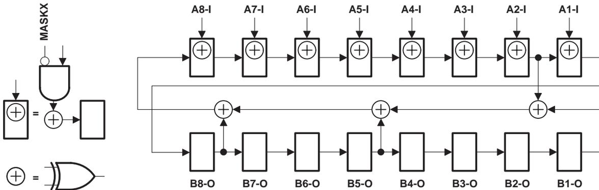
Figure 7. 16-Bit PSA Configuration (OEAB = 1, OEBA = 1)
