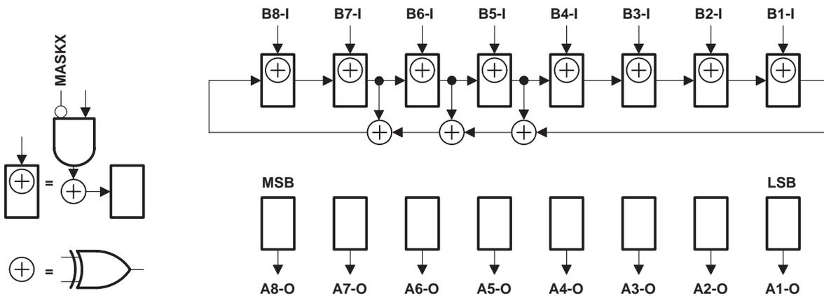
**Figure 12. 8-Bit PSA/COUNT Configuration (OEAB = 0, OEBA = 0)**
