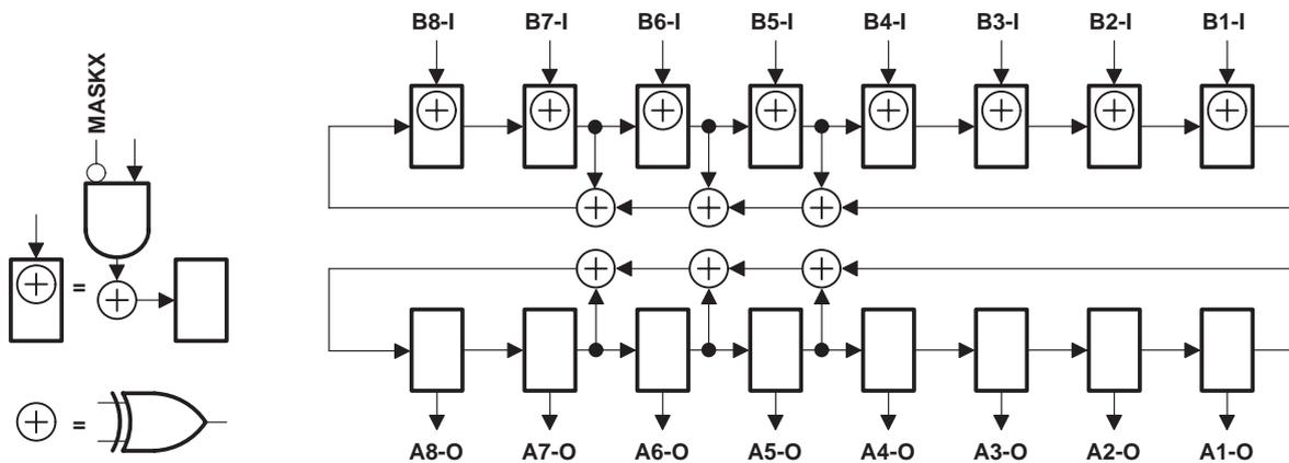
Figure 10. 8-Bit PSA/PRPG Configuration (OEAB = 0, OEBA = 0)
