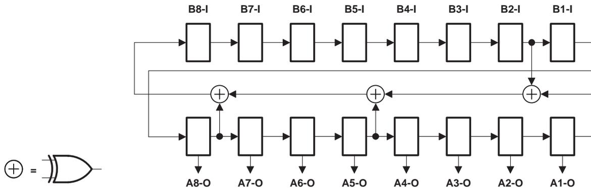
**Figure 6. 16-Bit PRPG Configuration (OEAB = 0, OEBA = 0)**
