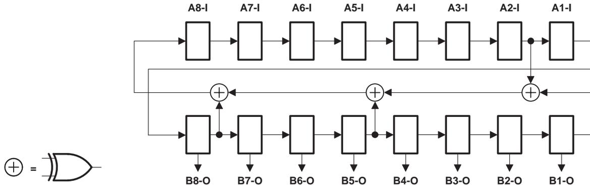
**Figure 5. 16-Bit PRPG Configuration (OEAB = 1, OEBA = 1)**
