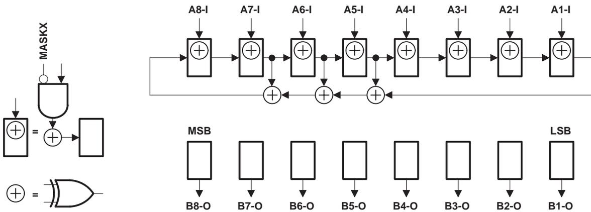
**Figure 11. 8-Bit PSA/COUNT Configuration (OEAB = 1, OEBA = 1)**
