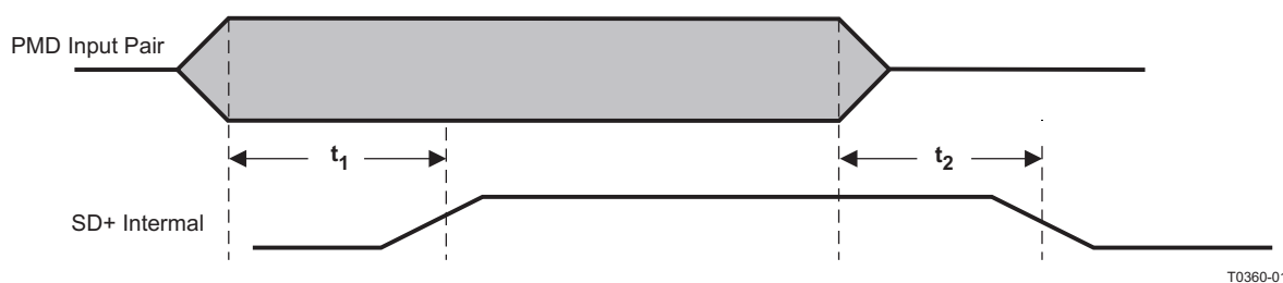
Figure 9-20. 100Base-TX Signal Detect Timing
