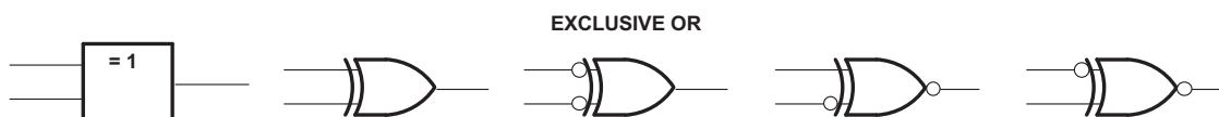
These are five equivalent exclusive-OR symbols valid for an SN74LVC1G86 gate in positive logic; negation may be shown at any two ports.
