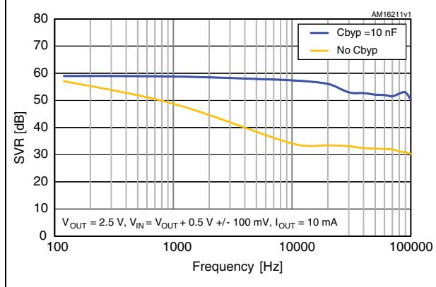
**Figure 22. SVR vs. frequency ( $V_O = V_{ADJ}$ )**
