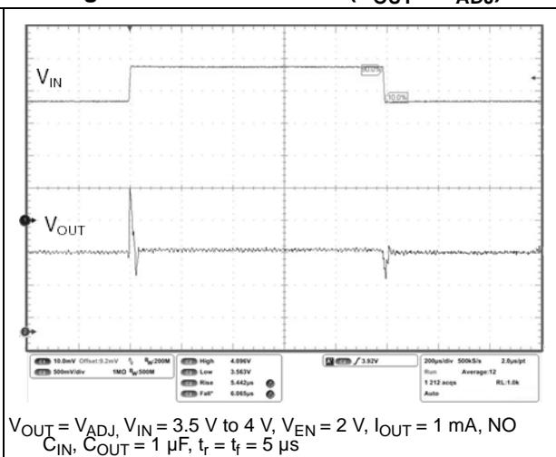
**Figure 28. Line transient ( $V_{OUT} = 3 \text{ V}$ )**
