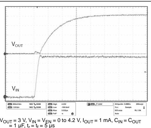
**Figure 32. Enable transient ( $V_{OUT} = V_{ADJ}$ )**
