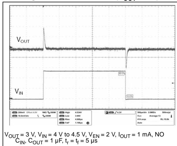
**Figure 29. Load transient ( $V_{OUT} = 3 \text{ V}$ )**
