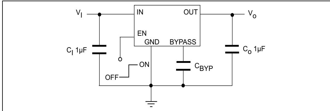
Figure 4. Typical application circuits for D version
