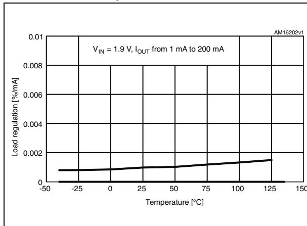
**Figure 13. Load regulation vs. temp. for fixed version**
