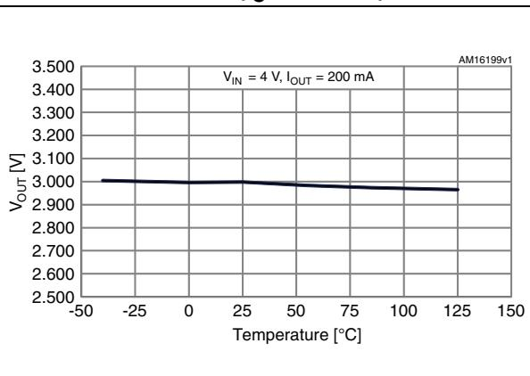
**Figure 10. Line regulation vs. temp. for adjustable version**
