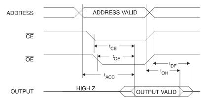
Notes: 1.  $\overline{\text{CE}}$  may be delayed up to  $t_{\text{ACC}}$  -  $t_{\text{CE}}$  after the address transition without impact on  $t_{\text{ACC}}$ .
