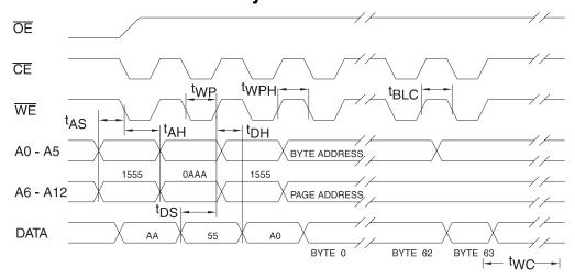
Notes: 1. A0 - A12 must conform to the addressing sequence for the first three bytes as shown above.
