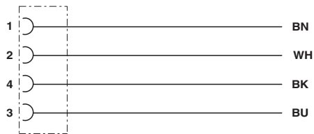
Contact assignment of the M12 socket
