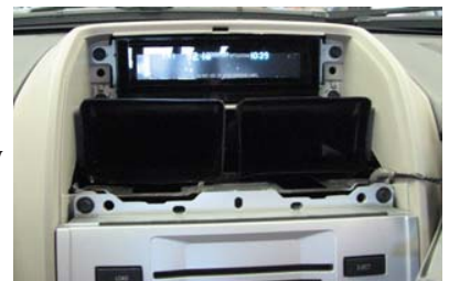
Air Vent Assembly Removed
