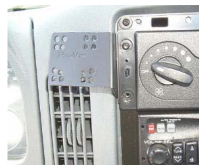
Install InDash on these (2) holes under climate control flange
