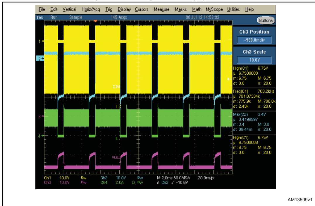
Figure 25: Inverting BB dimming operation
