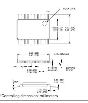
Datasheet of AT25320T2-10TI-2.7 - IC EEPROM 32KBIT 3MHZ 20TSSOP
