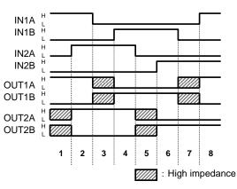
Fig.15 1-2 Phases Timing Sequence with IN/IN Input
