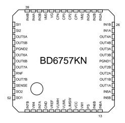
Fig.10 BD6757KN Pin Arrangement (Top View) UQFN52 Package
