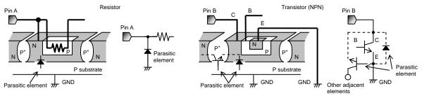
Fig.21 Example of Simple IC Architecture
