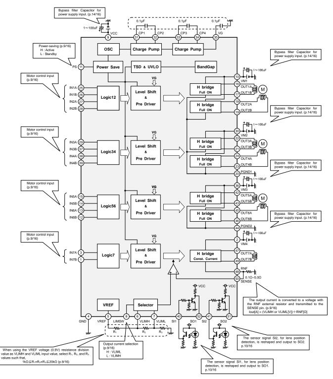
Fig.12 BD6757KN Application Circuit Diagram
