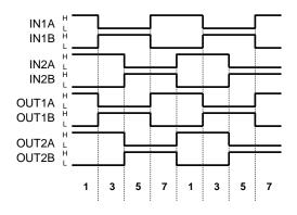
Fig.14 2 Phases Timing Sequence with IN/IN Input
