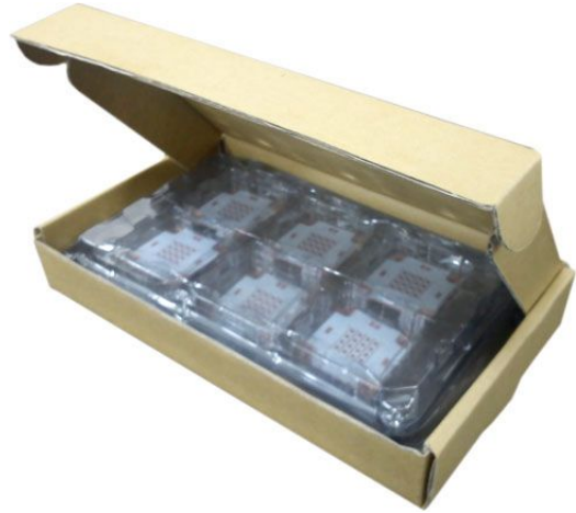
Fig. 6 - Tray and Box 5 Trays in One Anti-Static Bag, 2 Bags in One Carton, Contains 60 Pieces LED
