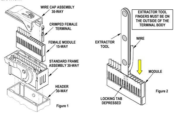
1. Insert the extractor tool into the module as shown in Figure 2.
