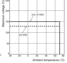
"Maximum Voltage" is the maximum voltage that can be applied to the relay coil. Note:
