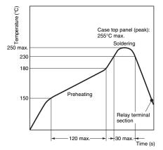
Note: The temperature profile indicates the temperature on the PCB.
